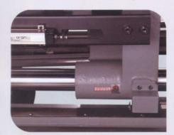
Adjustable rollers support the weight of mold and platen and distribute to all the area homogenously for long life operation.
