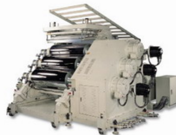
3 Roll stack at inclined configuration
